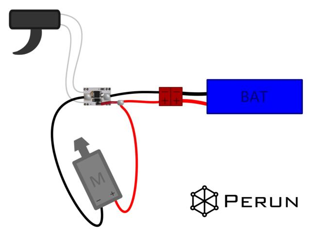
You may shorten the white and red cables already soldered to Perun AB as needed, but please do not replace them. After soldering the whole wiring together, use attached shrinktube for insulation.
